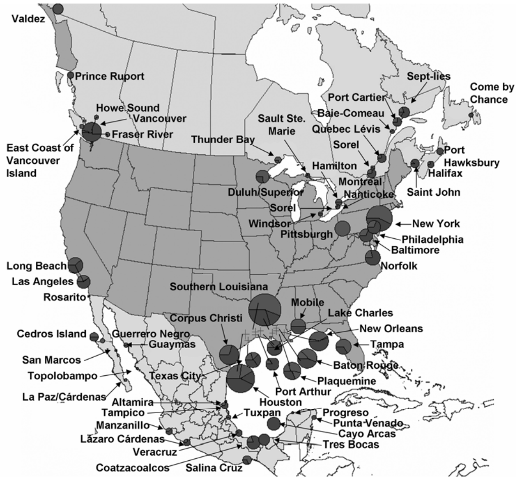
Fig. 37.4. Port freight traffic in North America (from U.S. Department of Transportation et al. 2000).
