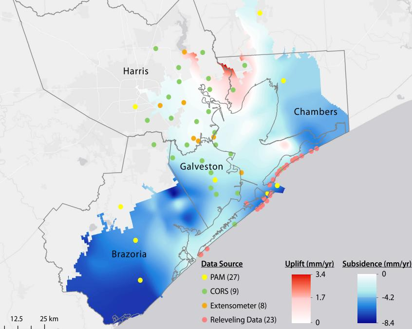
**Figure 1:** Final interpolated subsidence grid and location of data sources. PAM, CORS, and Extensometer data provided by the Harris Galveston Subsidence District. Releveling data from the National Geodetic Survey.
