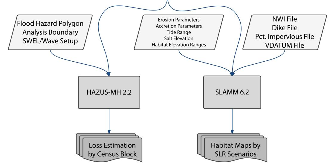
Figure 2: Inputs and outputs of the HAZUS-MH and SLAMM models used in this study.
